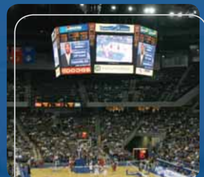
Qwest Center Omaha, Nebraska ProStar® 160x224 matrix 16.5 mm RGB and 112x160 matrix 23 mm RGB ProAd® 24x3328 matrix 23 mm RGB Custom LED scoreboard LED Auxiliary Scoring Display LED four-sided game clock/shot timer
