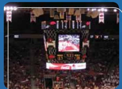
University of Arkansas Fayetteville, Arkansas ProStar® 224x288 matrix 10 mm RGB ProAd® 64x140 matrix 16.5 mm RGB ProAd® 48x1152 matrix 16.5 mm RGB BA-2002-4060-11 four-sided basketball scoreboard
