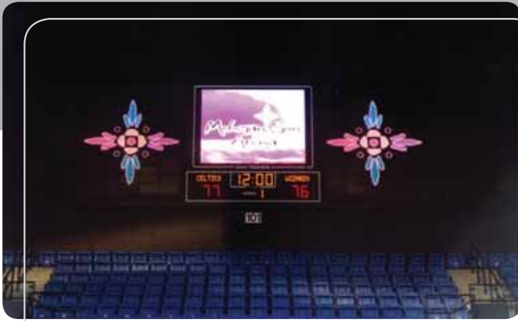
Mohegan Sun Casino Uncasville, Connecticut 192x240 matrix 12 mm RGB BB-2023-9 basketball scoreboard
